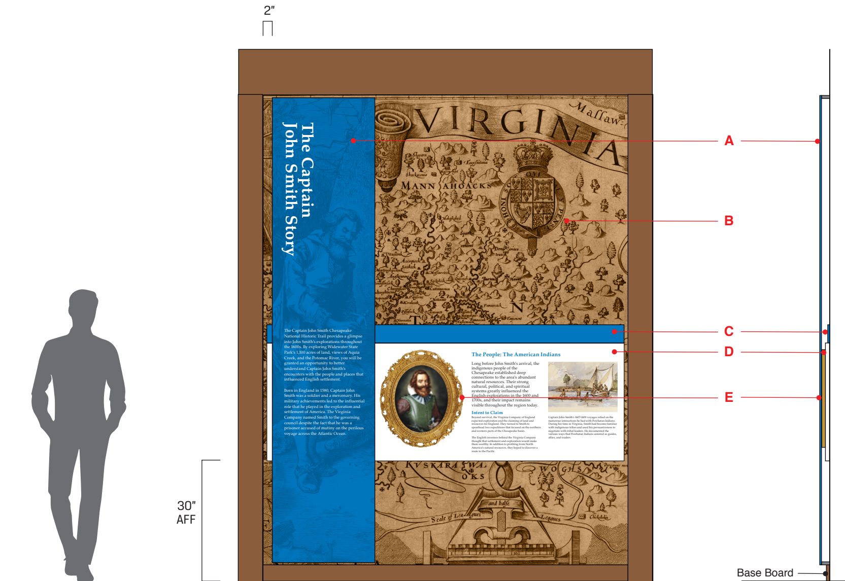
1 EXHIBIT BAY 1 Mounting Elevation SCALE: 1/2"=1'-0"
